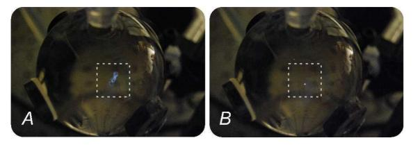
Figure 3: (A) Argon bubble moving in SA85 driving with the frequency associated with the first normal mode of a spherical resonator ( $f_0 = 29.2$ ) kHz. (B) Spatially fixed bubble due to the addition of a second component to the pressure field with a harmonic frequency ( $7f_0$ ). Both pictures were taken with a Nikon D50 camera, with a totally open diaphragm and with an integration time of 1 second Dellavale (2012). The concentration of dissolved gas in the liquid was equivalent to 16 mbar.
