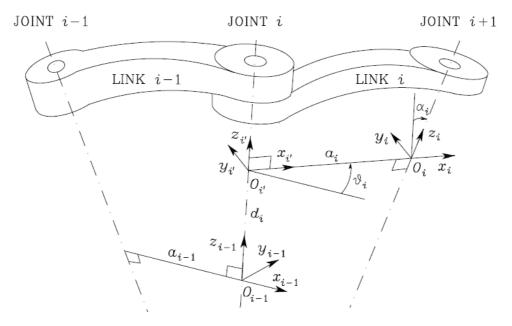
Figure 1: DH parameters. Figure by Sciavicco et al. (2009).
