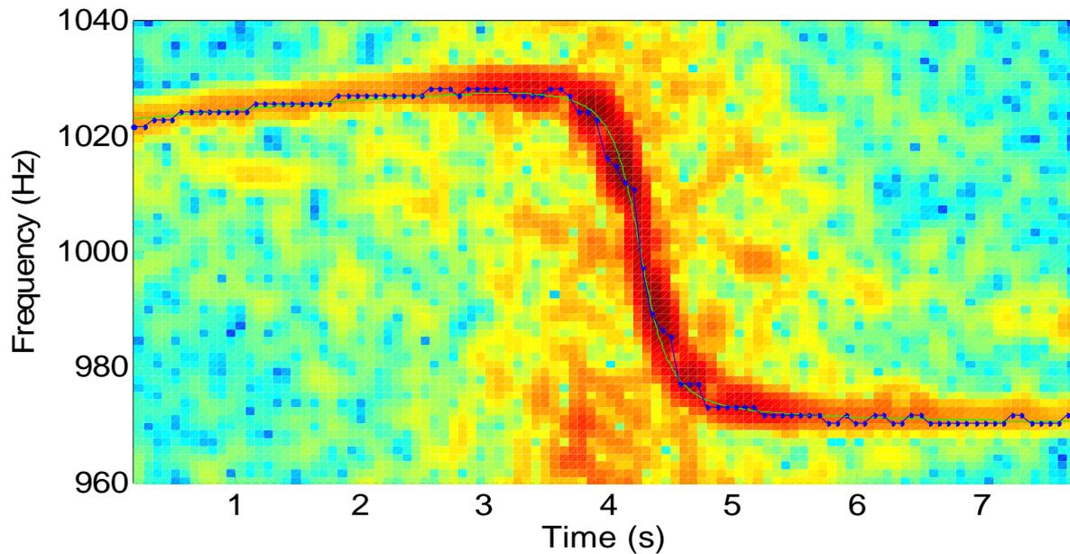
Figure 4: Input spectrogram around the pilot tone frequency, its maxima given by the ridge searching algorithm (dotted blue line) and its least squares fit (solid green line).
