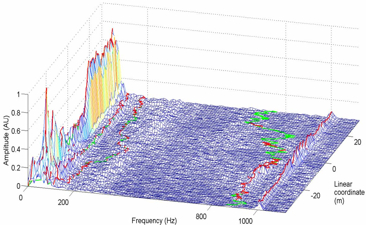
Figure 6: Spectrogram of the compensated signal and amplitude-position-frequency plot for each tone detected (solid lines). Low amplitude values for these tones are shown in green lines. Pilot tone information is included to illustrate the accuracy of the compensation algorithm proposed here.
